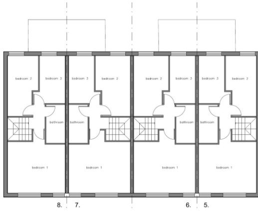
First Floor Plan Plot Floor Area = 48sqm
